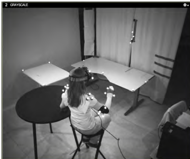
Figure 2: Optical tracking of the user and the actuated objects in the room is achieved with retro-reflective markers. This picture shows the view of one of the OptiTrack cameras.
