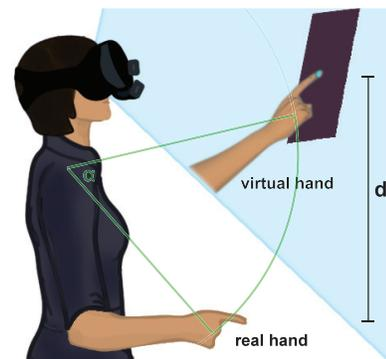
Figure 2. A VHS shift results in a vertical position offset  $d$  between the real and virtual hand. We arrive at this offset by translating the virtual hands on a circular path, based on a rotation ( $\alpha$ ) around the user's shoulder on the sagittal plane. To achieve a more realistic posture, the virtual forearm is always oriented towards the user's elbow.
